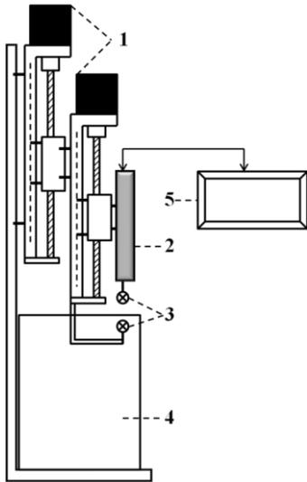
Fig. S1 The structure diagram of home-made instrument for detecting shrink force and peeling force. 1–lifting system; 2–pull/push dynamometer; 3–universal adjustable sample clamp; 4–temperature control system; 5–control panel.
