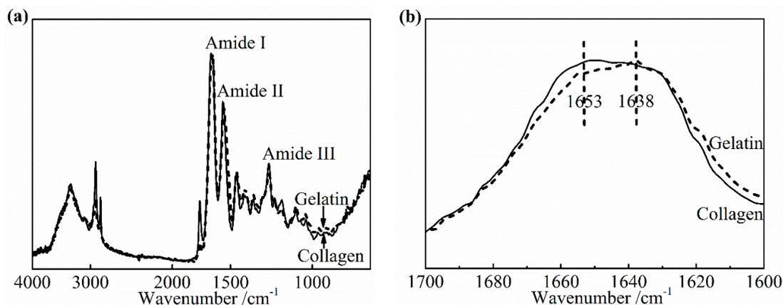
**Figure 8.** Fourier transform infrared spectroscopy (FTIR-ATR) spectra (a) and amide I band (b) of pure collagen film and gelatin film.
