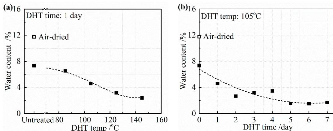
**Figure 7.** Water content in the collagen films after applying DHT treatment (a) at various DHT temperatures for 1 day and (b) at 105 °C for various DHT times.
