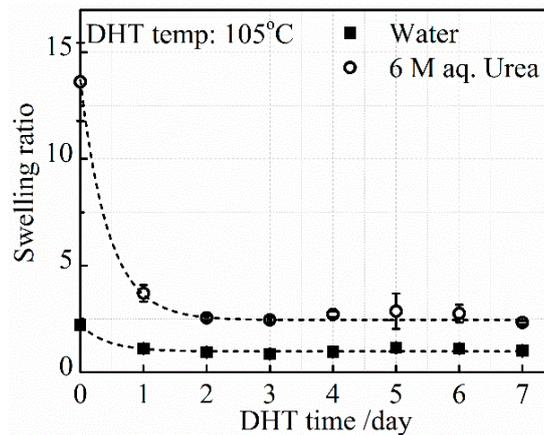
**Figure 6.** Change in  $SR_{urea}$  and  $SR_{water}$  with an increasing DHT time at 105 °C.
