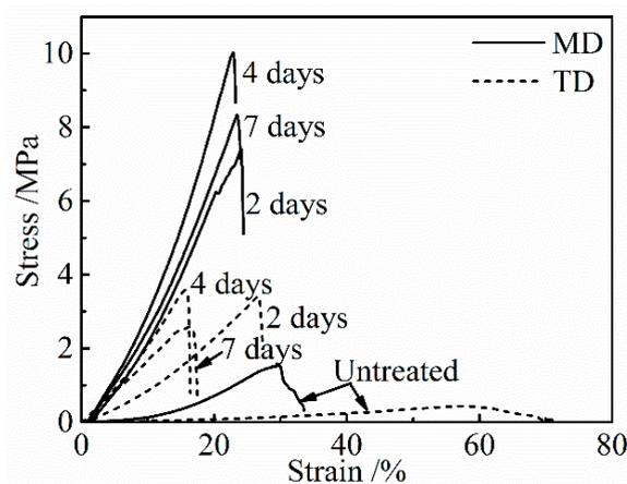
**Figure 3.** Stress-strain curves of the collagen films after applying DHT treatment for various DHT times at 105 °C.
