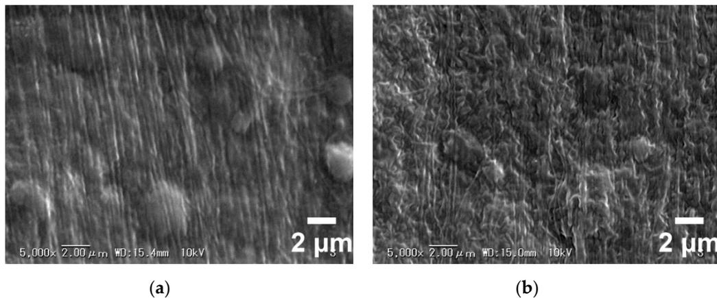
**Figure 13.** Scanning electron microscopy (SEM) images of (a) the untreated film and (b) the collagen film treated at 145 °C for 1 day.
