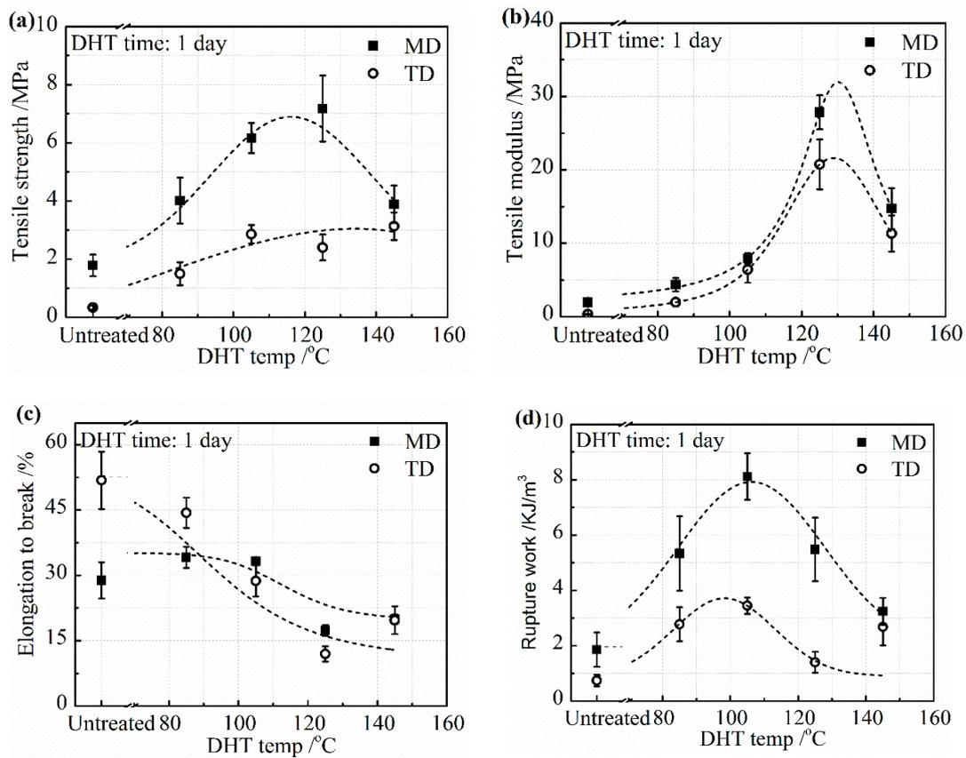
**Figure 2.** Mechanical properties: (a) tensile strength; (b) tensile modulus; (c) elongation to break; and (d) the rupture work of the collagen films after applying DHT treatment at various DHT temperatures for 1 day.
