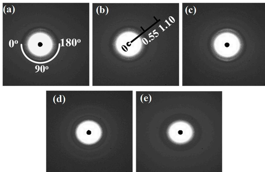
**Figure 11.** 2D SAXS patterns. The untreated film (a); collagen film treated at 105 °C for 3 days (b); 105 °C for 7 days (c); 125 °C for 1 day (d) and 145 °C for 1 day (e).
