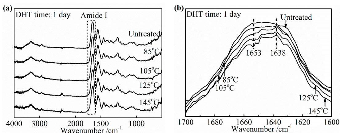
**Figure 9.** FTIR-ATR spectra (a) and amide I band (b) of the collagen films after applying DHT treatment at various DHT temperatures for 1 day.
