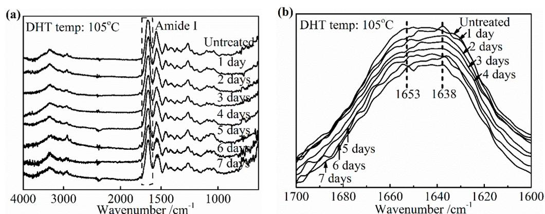
**Figure 10.** FTIR-ATR spectra (a) and amide I band (b) of the collagen films after applying a DHT treatment at 105 °C for various DHT times.
