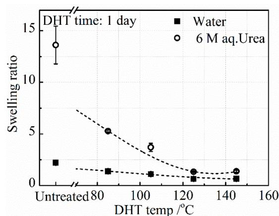
**Figure 5.** Change in  $SR_{urea}$  and  $SR_{water}$  with an increasing DHT temperature for 1 day.
