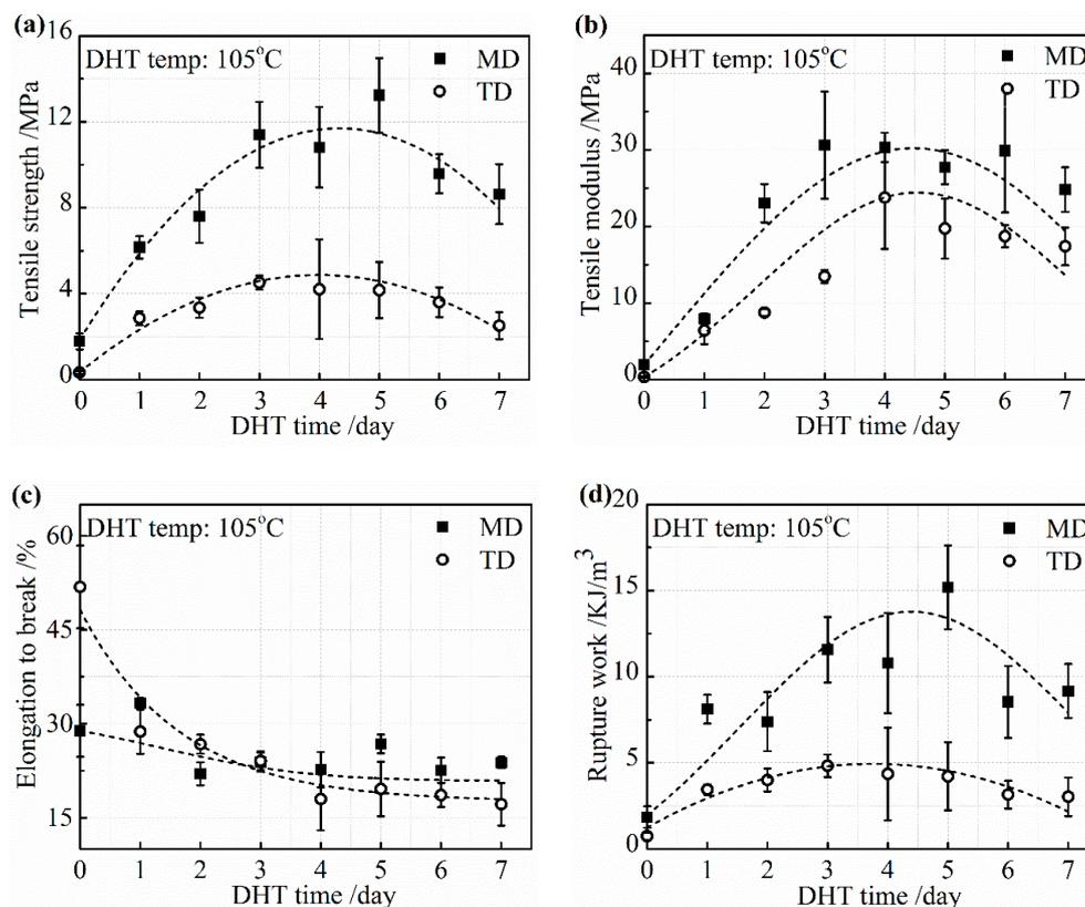
**Figure 4.** Mechanical properties: (a) tensile strength; (b) tensile modulus; (c) elongation to break; and (d) rupture work of the collagen films after applying DHT treatment at 105 °C for various DHT times.
