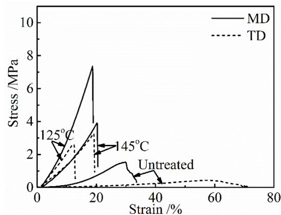
**Figure 1.** Stress-strain curves of the collagen films after applying the Dehydrothermal (DHT) treatment at various DHT temperatures for 1 day.
