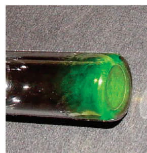
Figure 10. Photograph of slowly dried g -[PLA 200 - b -PnBA 200 ] (Table 2, entry 10) showing green color due to reflectance from the large self-assembled domains.
