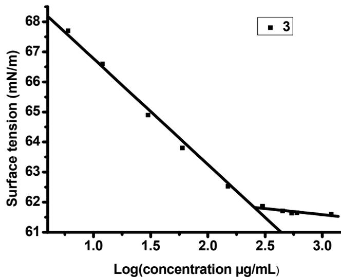
Solutions of **1**, **2** and **3** in water were made at the concentrations indicated in the figure. The vials were agitated gently overnight to promote the formation of micelles. The surface tension (mN/m) was measured for each solution. The surface tensions determined were plotted against the log of the concentration of **1**, **2** and **3**. The inflection point as determined by the best fit of the data yielded CMC's of 0.18 mg/mL for **1**, 0.2 mg/mL for **2** and 0.25 mg/mL for **3**.
