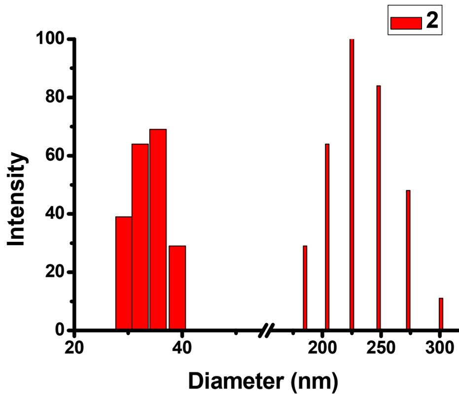
Dynamic Light Scattering of 1 mg/mL of **2** in water shows hydrated monomer scattering at 33.7 nm in diameter with an average polydispersity of 0.08 and micelle of mean diameter 232.6 nm with an average polydispersity of 0.12.
