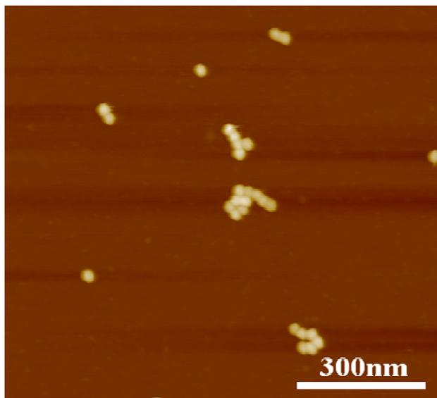
AFM image of gold NPs with thiol-mPEG (5KDa) after removing excess PEG. Individualized NPs are stable only in the presence of excess thiol-mPEG, and indeed, if the excess of the thiol-mPEG is removed by centrifugation, the solution of NPs become unstable, forming aggregates.
