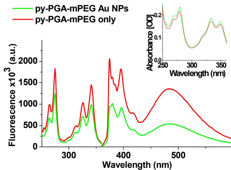
The intensity of pyrene adsorbance is dampened due to perturbations of gold nanoparticles, suggesting direct interaction of pyrene with the gold surface<sup>[5, 7]</sup>.
