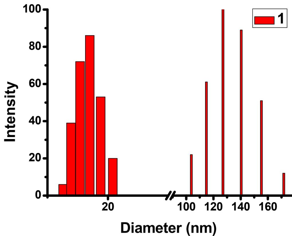
Dynamic Light Scattering of 1 mg/mL of **1** in water shows hydrated monomer scattering at 16.7 nm with an average polydispersity of 0.095 and micelles with mean diameter of 132.7 nm with an average polydispersity of 0.12.
