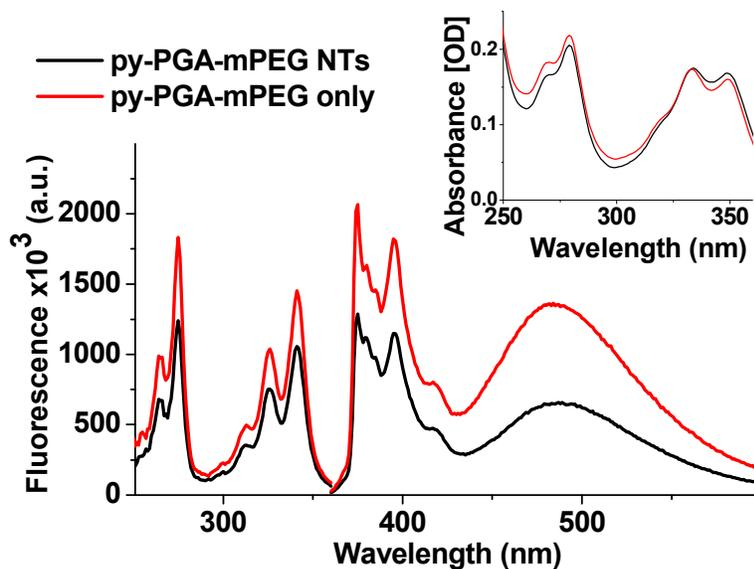
While PMHC<sub>18</sub> likely interacts with the SWNT sidewall via van der Waals' and entropic forces, the pyrene moiety has been reported to demonstrate a strong tendency to adsorb on SWNTs by  $\pi$ -stacking and hydrophobic interactions in aqueous media<sup>[2-5,6]</sup>. Proof of the intimate interaction between pyrene and the NT sidewall was observed by quenching of pyrene fluorescence relative to free pyrene-containing methoxyPEG- $\gamma$ PGA at the same OD.
