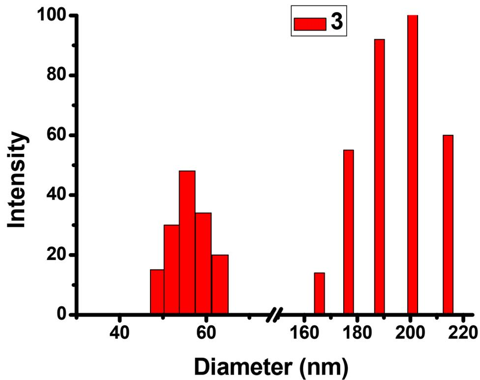
Dynamic Light Scattering of 1 mg/mL of **3** in water shows hydrated monomer scattering of 56.1 nm in diameter with an average polydispersity of 0.08 and mean micelle diameter of 196.3 nm with an average polydispersity of 0.09.
