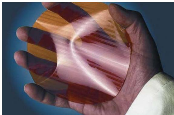
**Fig. 15** ORMOCER<sup>®</sup> waveguides on a flexible foil.
