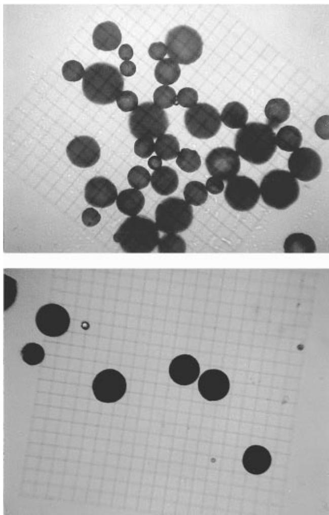
**Figure 1**—Optical micrographs of the gelatin nanoparticle–PLGA microsphere composites: (A, top) prepared by the phase separation method and (B, bottom) prepared by the solvent extraction method.
