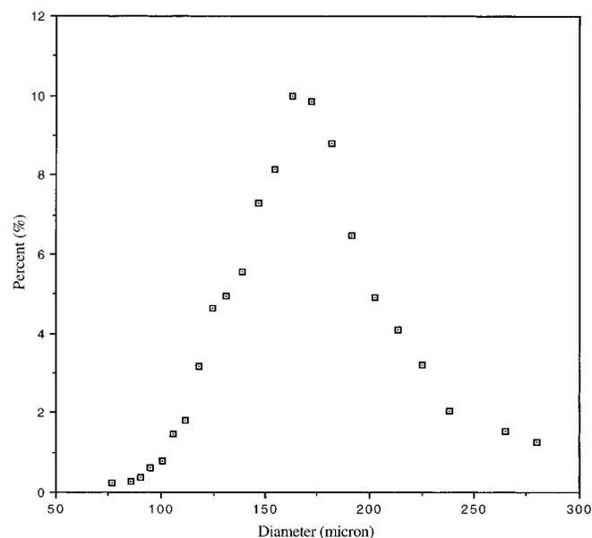
**Figure 2**—Size distribution of the gelatin nanoparticle–PLGA microsphere composites: (A, top) prepared by the phase separation method and (B, bottom) prepared by the solvent extraction method.
