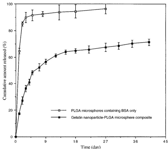
**Figure 3**—In vitro release of BSA from the gelatin nanoparticle-PLGA microspheres composite and the PLGA microspheres containing only BSA, prepared by the phase separation method.
