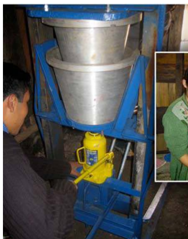
Clay pots, made in a press such as the one shown here (left) in a Guatemalan factory, fit inside plastic buckets for filtering water.
