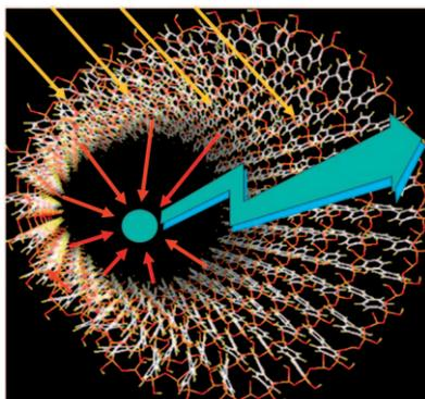
**Light aqueduct:** Periodic mesoporous organosilica exhibit strong light absorption due to densely packed organic chromophores within the pore walls. Light energy absorbed by 125 biphenyl groups in the pore walls is funneled into a single coumarin 1 molecule in the mesochannels with almost 100% quantum efficiency, and results in significant enhancement of emission from the coumarin 1 dye.
