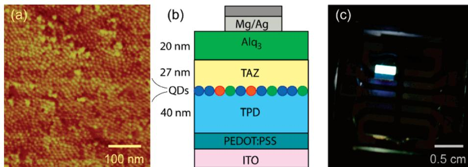
**Figure 1.** (a) Atomic force microscope phase image of blue QDs forming approximately 1.1 monolayers on top of a 40 nm thick TPD film. (b) Device cross section of a white QD-LED. (c) Photograph of a white QD-LED in operation with 10 V of applied forward bias.
