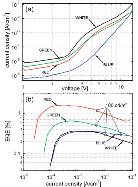
**Figure 3.** Current–voltage characteristics (a) and external electroluminescence quantum efficiency (b) measured for red, green, blue, and white QD-LEDs labeled with red, green, blue and black lines, respectively. The circled data points indicate device brightness of 100 cd/m<sup>2</sup>.
