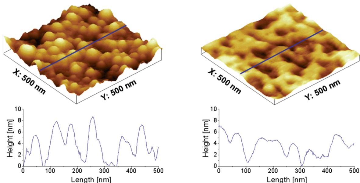
**Figure 5.** Atomic force microscope (AFM) height image and surface profile of a film prepared from dispersion 2\_1D49 before (left) and after annealing (right) at 150 °C.
