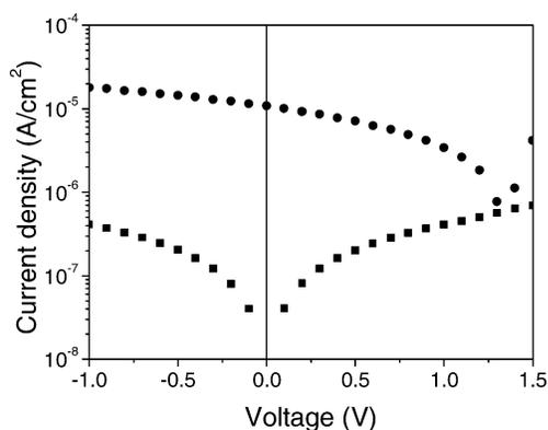
**Figure 10.**  $I(U)$  characteristics for a particle blend device containing 43 nm PFB particles and F8BT particles (blend ratio 1:2) in the dark (squares) and under white light illumination (circles) with an intensity of 100 mW/cm<sup>2</sup>.
