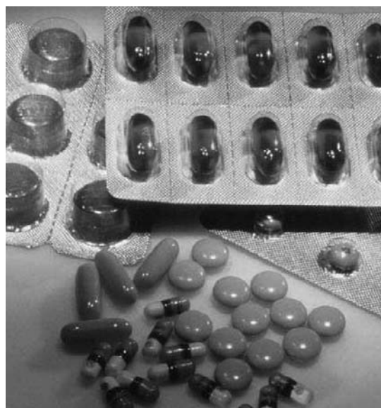
Figure 16 Packaging of drugs with barrier films from PCTFE. Courtesy Honeywell.
