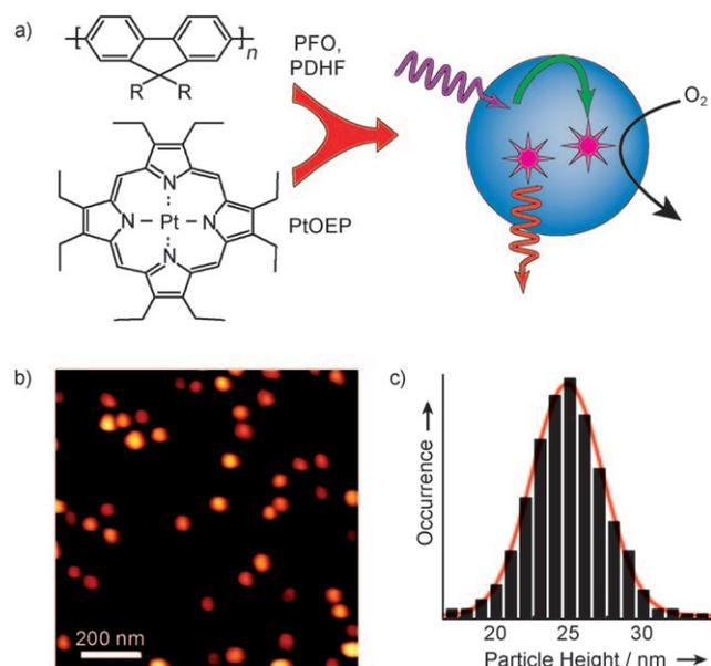
**Figure 1.** a) Schematic illustration of the formation of conjugated polymer dots for oxygen sensing. b) Representative AFM image of PtOEP-doped PDHF dots dispersed on a mica substrate. c) Histogram of particle-height data obtained from the AFM image in (b).
