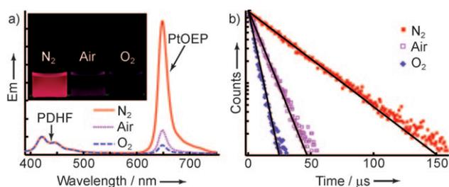
**Figure 3.** a) Oxygen-dependent emission spectra of the 10% PtOEP-doped PDHF dots (excitation wavelength = 350 nm). The inset shows doped PDHF dots in aqueous solutions saturated with nitrogen, air, and oxygen, respectively, under a UV lamp. b) Phosphorescence decays of the 10% PtOEP-doped PDHF dots with different oxygen concentrations. The scattered symbols represent experimental data, and the solid lines are fits.
