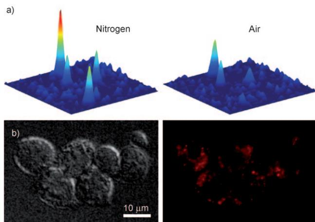
**Figure 4.** a) Single-particle phosphorescence images of the doped CPdots immobilized on a coverslip under a nitrogen and an air atmosphere, respectively. b) DIC and phosphorescence images that indicate uptake of the nanoparticle sensor by macrophage cells.
