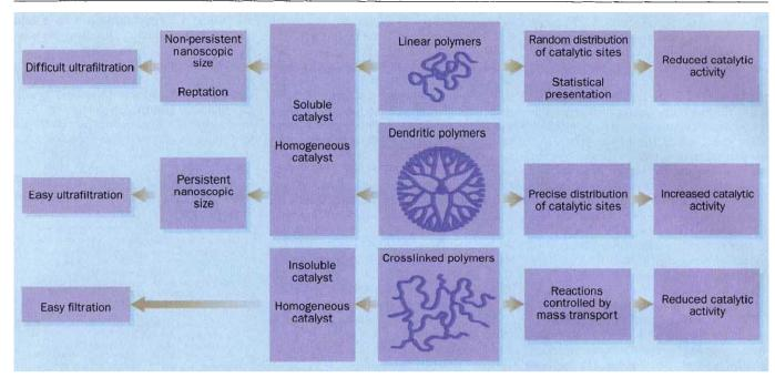
The benefits of branching — schematic illustration of the three main types of polymer catalysts, together with their distinguishing properties and functional characteristics. The properties to the left of the
