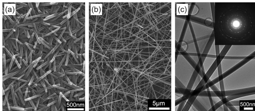
**Figure 2.** FE-SEM (A,B) and TEM (C) images of the binary nanostructures with a TPP/rubrene molar ratio of 100:1 prepared under different conditions. Inset: SAED pattern of the nanowires.
