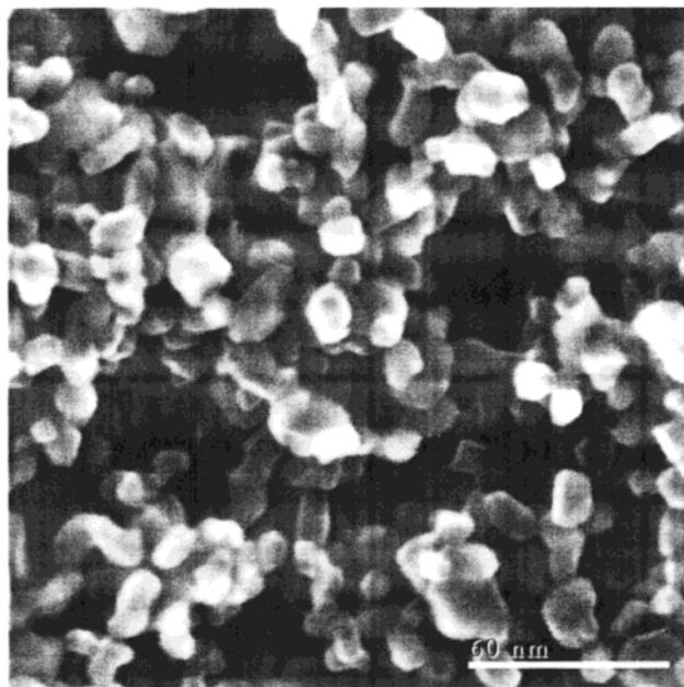
FIGURE 1. Scanning electron microscope pattern of a typical nanocrystalline TiO<sub>2</sub> film.
