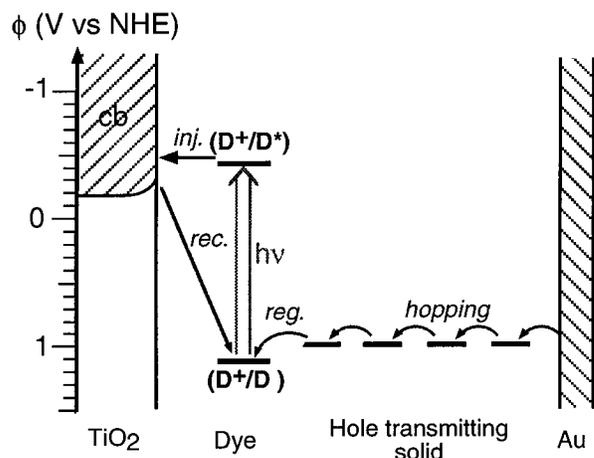
**FIGURE 3.** Dye-sensitized heterojunction solar cell where the electrolyte in Figure 1 is replaced by an organic hole conductor. Energy levels of the different redox species and  $\text{TiO}_2$  vs NHE are shown. Electron-transfer reactions are symbolized by black arrows.
