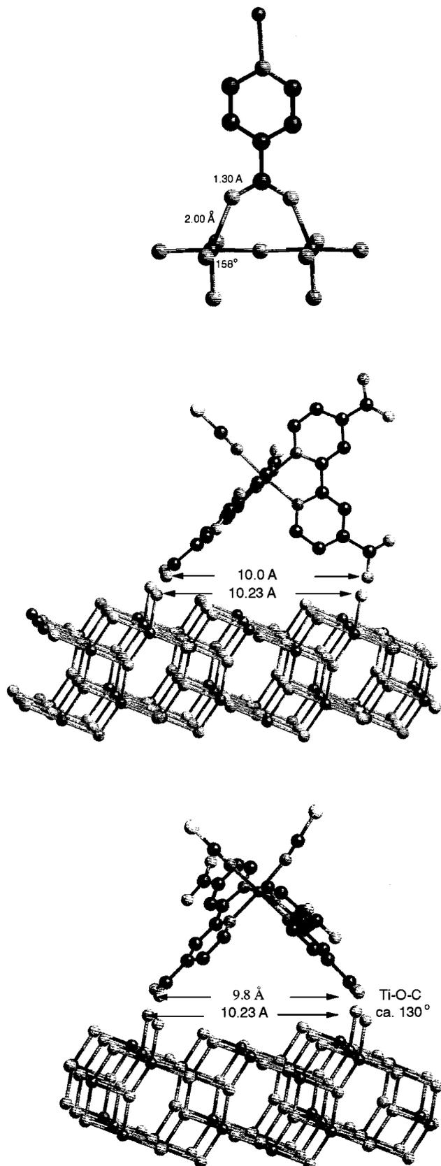
**FIGURE 5.** Anchoring of the N3 dye on the (101) surface of anatase.  $-NCS$  groups may play an important role in this process. The  $-NCS$  groups point in the direction of the electrolyte, which may facilitate reduction by  $I^-$ , making it particularly suitable for highly efficient solar cells. The LUMO in Figure
