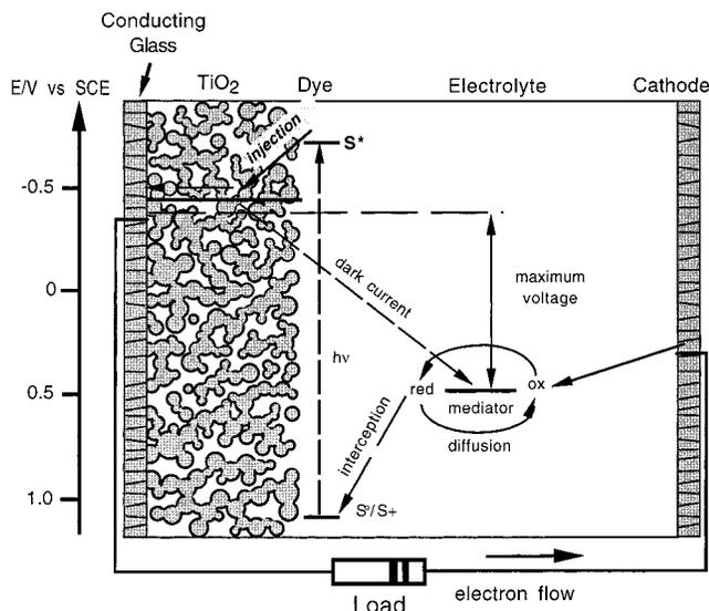
**FIGURE 2.** Schematic representation of the principle of the nanocrystalline injection cell to indicate the energy level in the different phases. The cell voltage observed under illumination corresponds to the difference in the quasi-Fermi level of the  $\text{TiO}_2$  under illumination and the electrochemical potential of the electrolyte. The latter is equal to the Nernst potential of the iodide/triiodide redox couple used to mediate charge transfer between the electrodes.
