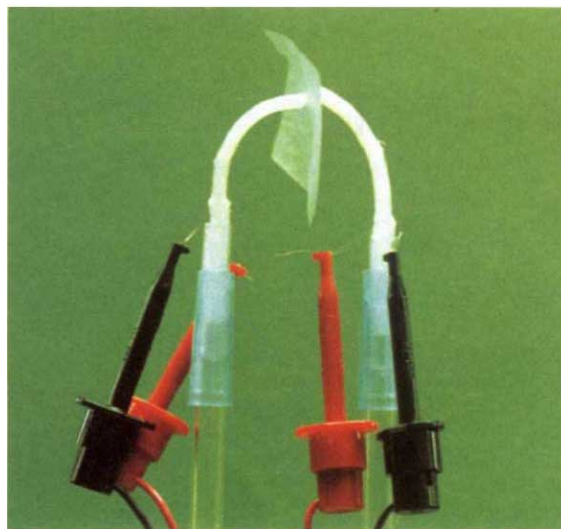
Gripping stuff: the newest polymer-gel fingers grasp a piece of paper at the recent RoboBug Fest.
