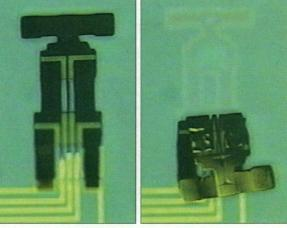
**Soft robots.** Microtools operating with the help of conjugated polymer actuators (9). The microrobotic arm has three separately controlled joints (see inset)—finger, wrist, and
