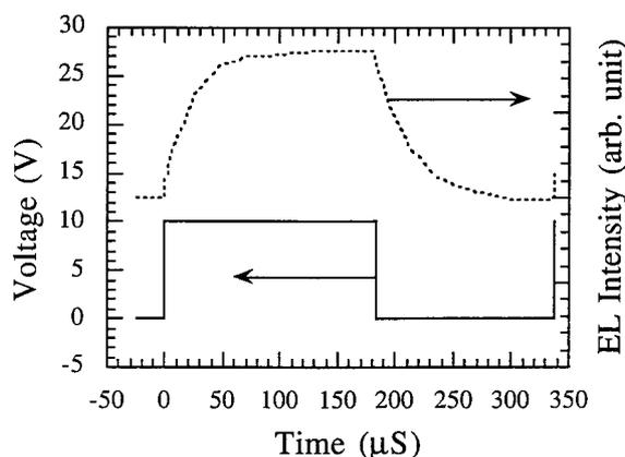
Fig. 4. Transient response of a BuEH-PPV/CE/Li<sup>+</sup> LEC.
