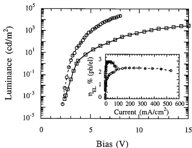
Fig. 3. *L-V* in two frozen-junction LECs with different blend ratios (circles: BuEH-PPV/CE/Li triflate/OCA = 1:1:0.2:0.1; squares: BuEH-PPV/CE/Li triflate = 2:1:0.2). Their corresponding external quantum efficiencies are shown in the inset.
