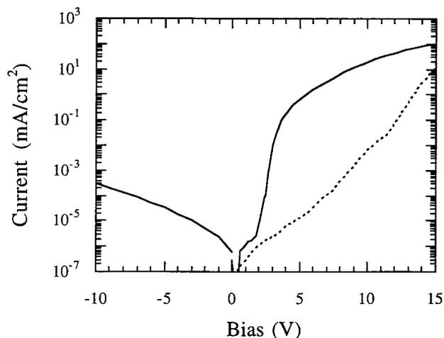
Fig. 2. *I-V* characteristics of a BuEH-PPV/CE/Li<sup>+</sup> LEC in pristine condition (dotted line) and with frozen p-i-n junction (solid line).
