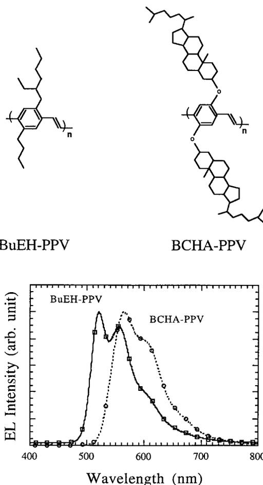
Fig. 1. Chemical structures (top) and electroluminescent spectra (bottom) of BuEH-PPV and BCHA-PPV.
