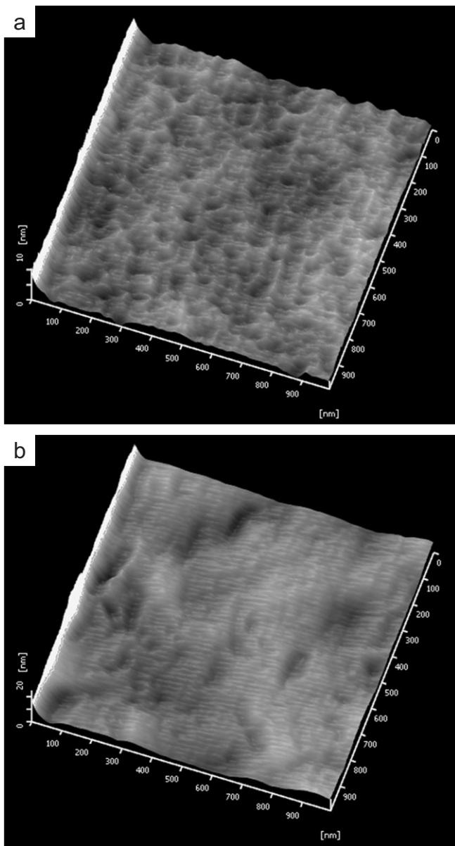
**Figure 5.** AFM images ( $1\ \mu\text{m} \times 1\ \mu\text{m}$  scale) of the PFO-R005-G010 copolymer film a) before and b) after heat treatment at  $150\ ^\circ\text{C}$  for 10 min.
