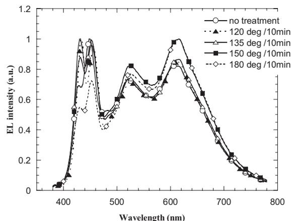
**Figure 3.** EL spectra of the white-EL device with different thermal treatments.
