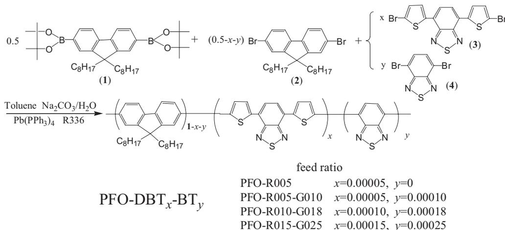
**Scheme 1.** Chemical structures and synthetic route for the formation of the copolymers.
