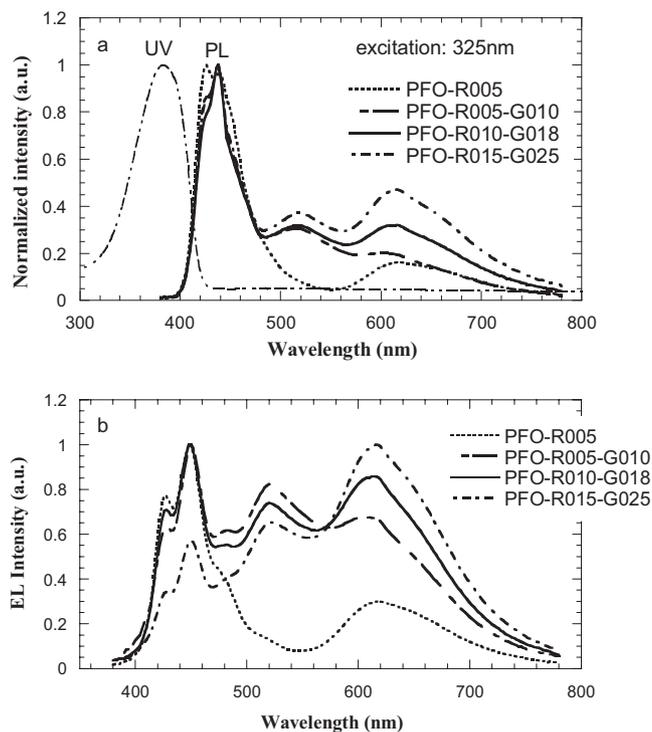
**Figure 1.** a) UV absorption and PL spectra of the copolymers. b) Electroluminescence (EL) spectra of the devices made from these copolymers with device configurations ITO/PEDOT/PVK/PFO-BT-DBT/Ba/Al at a current density of 13.3 mA cm<sup>-2</sup>. PVK: poly(vinylcarbazole).
