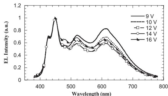
**Figure 2.** EL spectra of the devices with the PFO-R010-G018 copolymer at voltages varying from 9 to 16 V.
