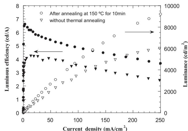
**Figure 4.** Luminous efficiency and light output versus the current density of devices manufactured from the copolymer PFO-R010-G018 film with and without thermal treatment (at 150 °C for 10 min) before cathode deposition.
