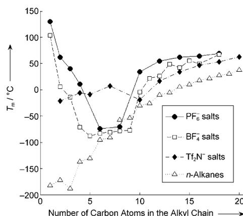
**Figure 1.** Influence of alkyl-chain length on  $T_m$  in *N*-alkyl *N*-methylimidazolium salts and the corresponding *n*-alkanes. The graph includes data from the literature<sup>[4–9]</sup> and newly synthesized ionic liquids.
