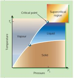
Critical conditions: above, phase diagram for a pure substance showing the critical pressure,  $P_c$ , and temperature,  $T_c$ . Above right, the effect of heating CO<sub>2</sub> rapidly through the critical point from liquid (top) to supercriticality (bottom).
