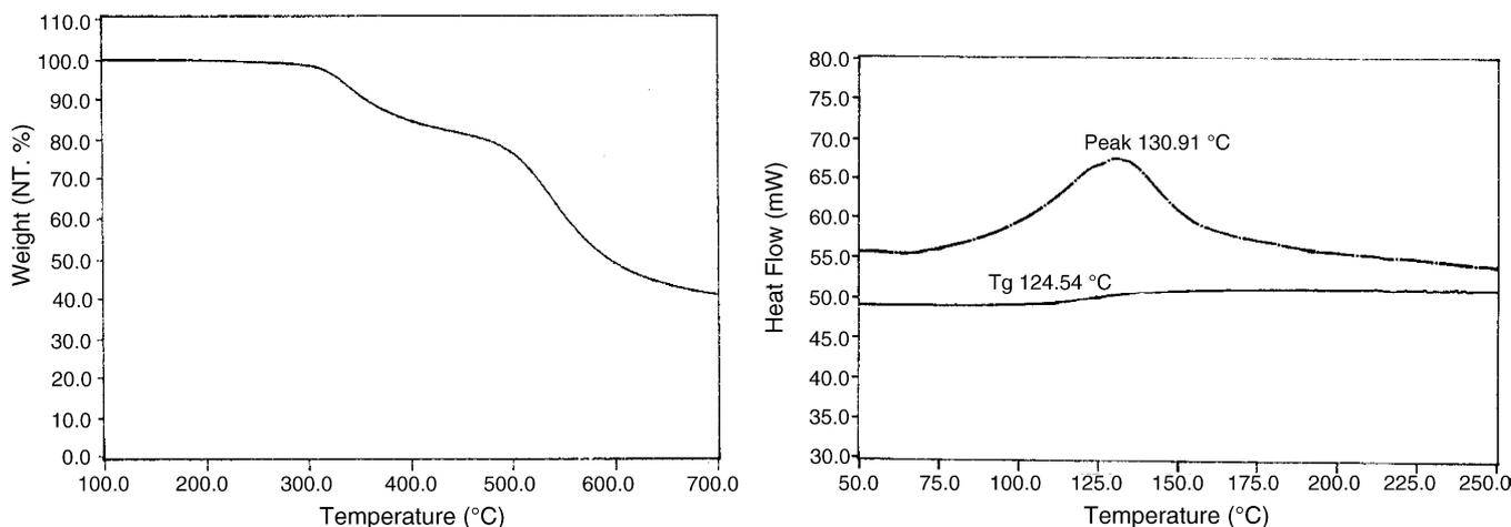
Fig. 4. (a) TGA of copolymer **8b** (1100 equiv. weight) in nitrogen (10 °C min<sup>-1</sup>). (b) DSC of Copolymer **8b** (1100 equiv. wt.) at 10 °C min<sup>-1</sup> showing first and second heating curves.
