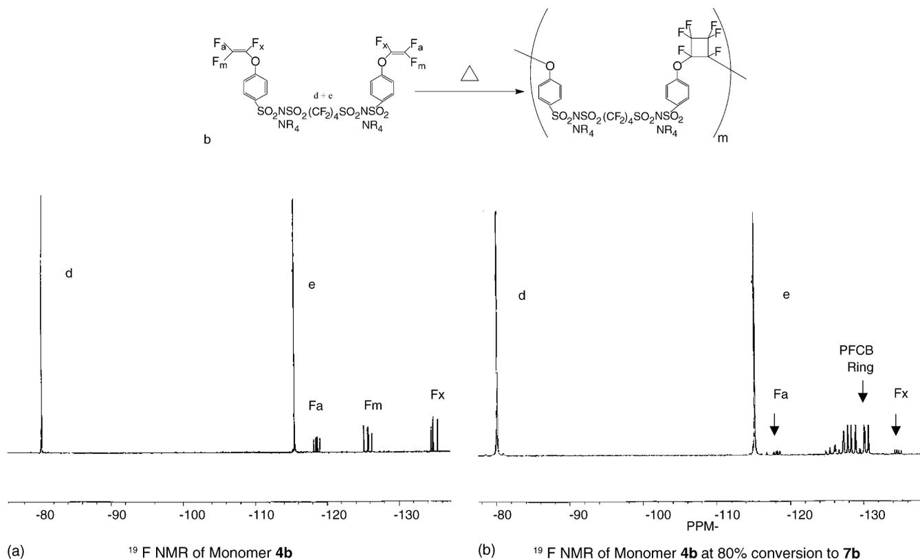
Fig. 3. (a)  $^{19}\text{F}$  NMR of monomer **4b**. (b)  $^{19}\text{F}$  NMR of monomer **4b** at 80% conversion to **7b**.
