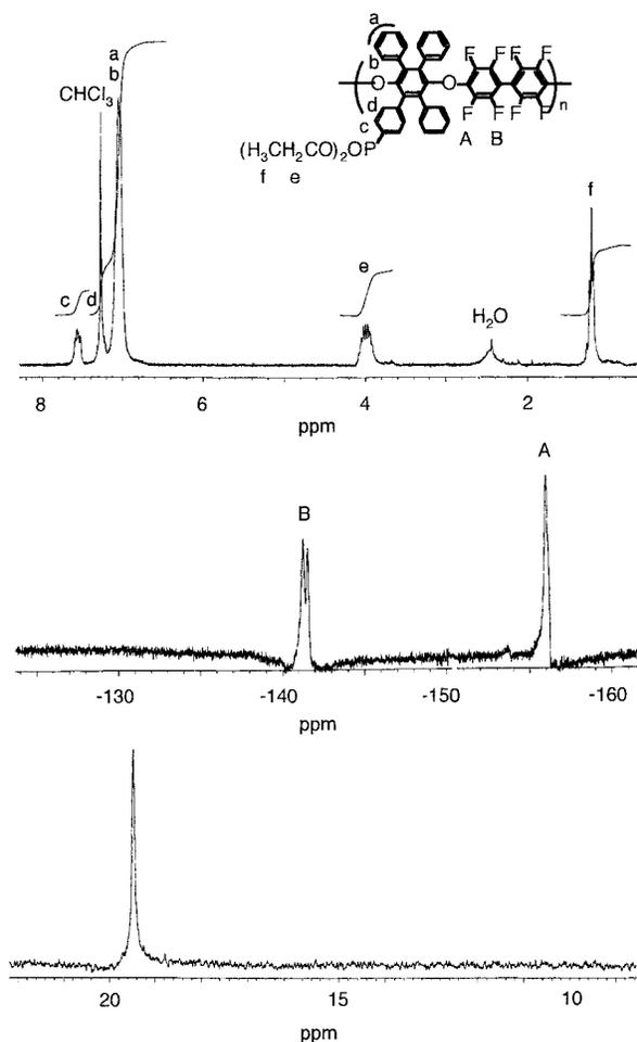
**Figure 1.**  $^1\text{H}$  (top),  $^{19}\text{F}$  (middle), and  $^{31}\text{P}$  (bottom) NMR spectra of **8a**.
