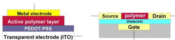
Fig. 1. Schematic representations of a two-terminal photovoltaic device (left) and a three-terminal transistor (right).
