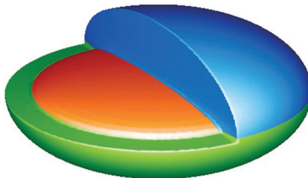
Figure 1. Representation of a disk-shaped Janus micelle. Complex coacervate core (PAA and P2MVP): orange; coronal hemispheres: green (PEO) and blue (PAAm).
