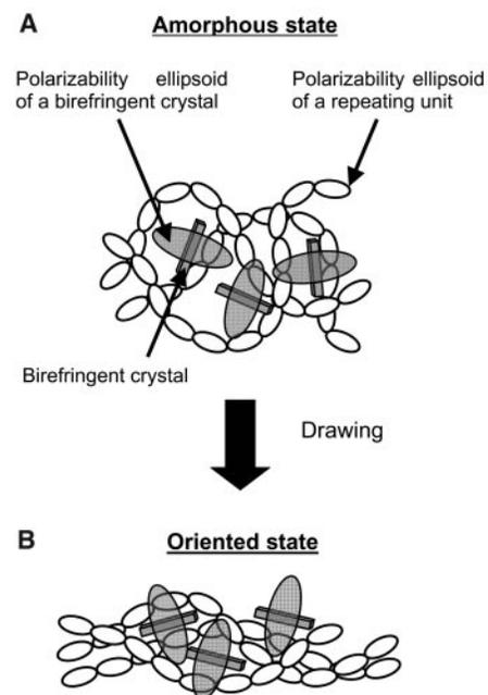
**Fig. 1.** Mechanism for the compensation of orientational birefringence by the birefringent crystal dopant method. (A) In the completely amorphous state, polymer chains and birefringent crystals are randomly oriented, so that the polymer containing the birefringent crystals exhibits no birefringence. (B) Polymer chains and birefringent crystals are oriented in the drawing direction. However, birefringence of the polymer is compensated by that of the crystal.
