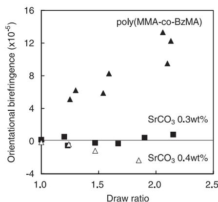
**Fig. 3.** Orientational birefringence of the poly(MMA-co-BzMA) films containing  $\text{SrCO}_3$  with respect to draw ratio.
