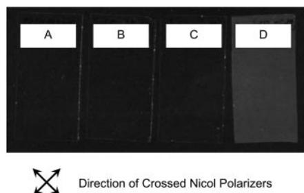
**Fig. 2.** A photograph of polymer films placed between crossed Nicol polarizers. (A) Poly(MMA-co-BzMA), (B) containing 0.5 wt %  $\text{SrCO}_3$  with a length of 200 nm and a width of 20 nm, (C) containing 1.0 wt %  $\text{SrCO}_3$  with a length of 200 nm and a width of 20 nm, and (D) containing 0.5 wt %  $\text{SrCO}_3$  with a length of 3.0  $\mu\text{m}$  and a width of 300 nm.
