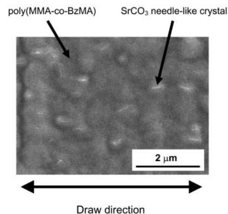
**Fig. 4.** A photograph of the heat-drawn poly(MMA-co-BzMA) film containing 1.0 wt %  $\text{SrCO}_3$ . Draw ratio = 2.0; drawing temperature = 130°C; drawing speed = 4 mm/min.
