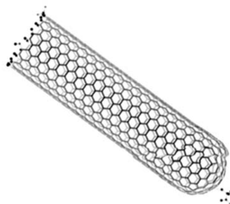
Figure 3. Derivatized section of a (10,10) fullerene nanotube with one end open.
