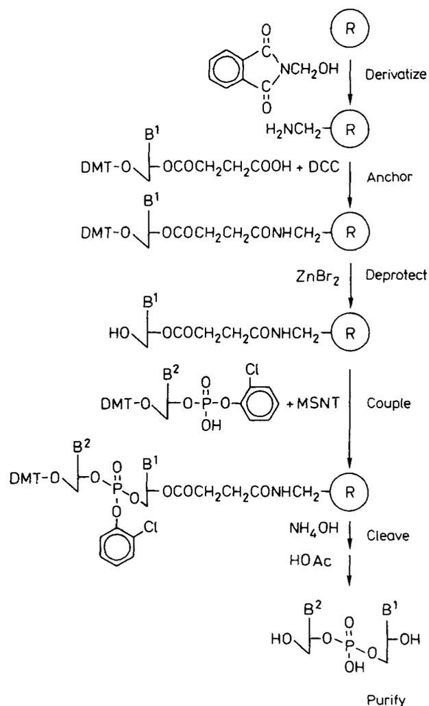
Fig. 4. Scheme for solid phase nucleotide synthesis (see text).
