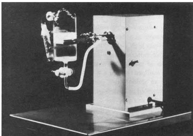
Fig. 6. Manually operated apparatus for peptide synthesis.
