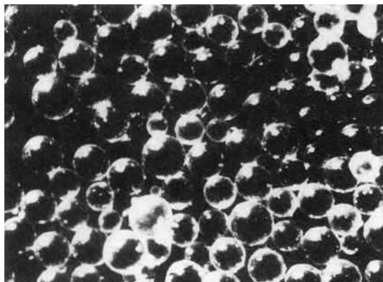
Fig. 5. Copolymer of styrene and divinylbenzene (1%). Top: structural formula. Bottom: photomicrograph of the resin beads.
